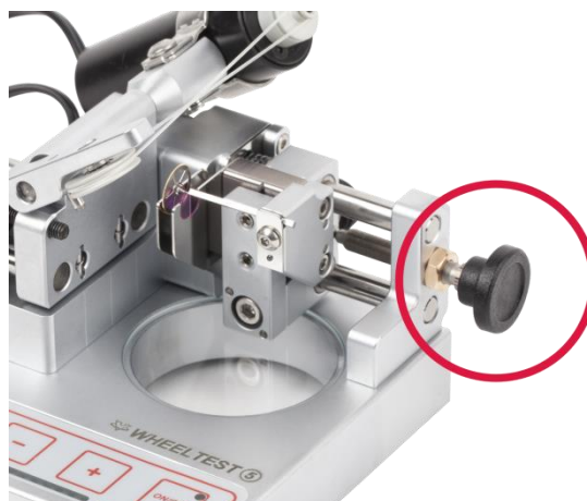
Figure 5: Micrometer screw for adjusting the distance between the two « V's »
