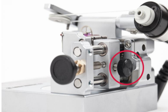
Figure 6: « V's » height adjustment screw
