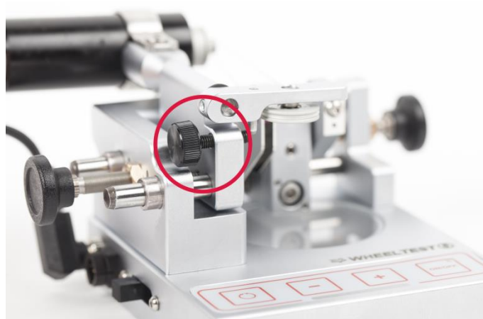
Figure 9: Screw to adjust the belt stop
