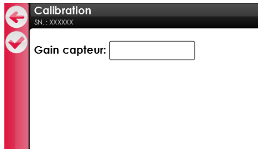
Figure 40: Calculated gain and validation before saving to the sensor
