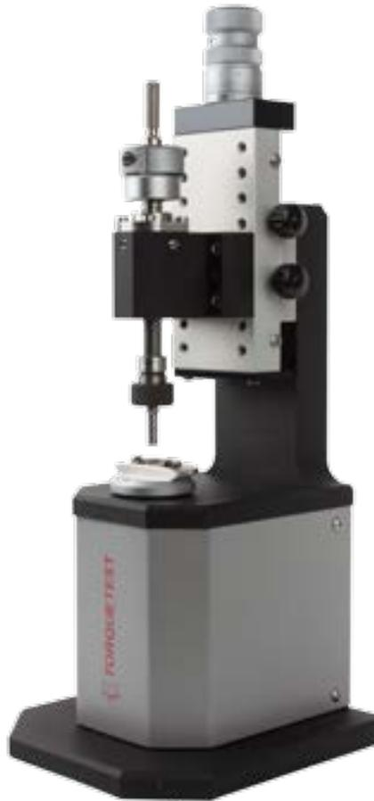
TORQUETEST is compatible with the VISIOTEST display unit. VISIOTEST automatically identifies the measurement scale selected. Measured values can be stored onto an SD card, exported via a USB connection or printed on tickets. VISIOTEST has an embedded statistical module for in depth analysis.
