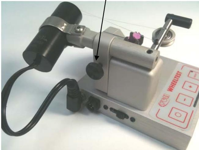
**Figure 6: Adjustment of the axial position of the motor**
