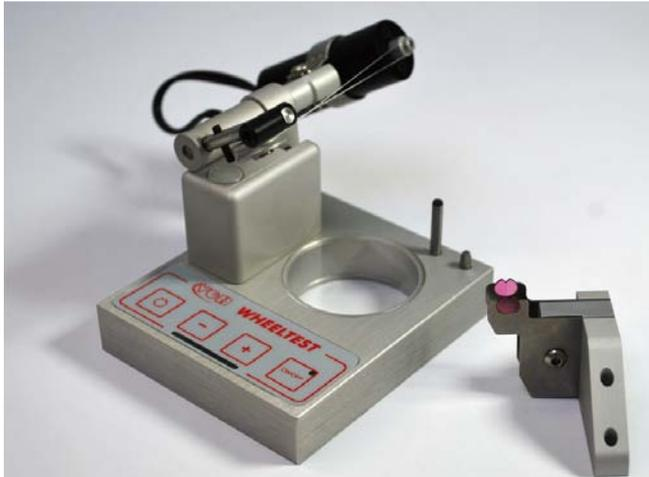
Figure 2: Wheeltest III with a set of specific jaws
