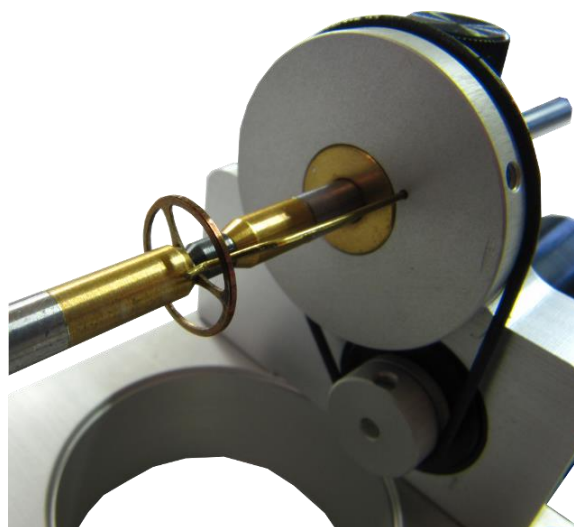
Figure 2: correct positioning of the wheel
